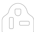
Power cord with plug (NEMA 6-20P)
