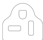
Power cord with plug (NEMA 5-20P)
