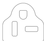
Power cord with plug (NEMA 6-20P)
