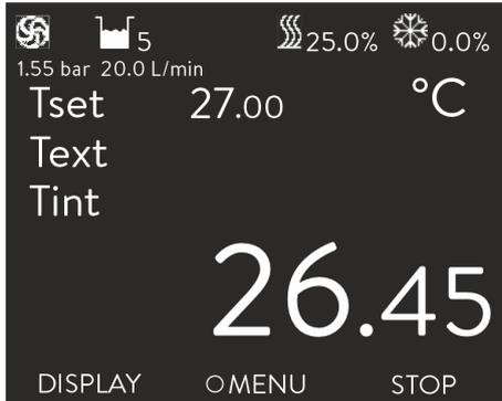
Fig. 9: Basic windows Integral XT and Integral P with flow controller
