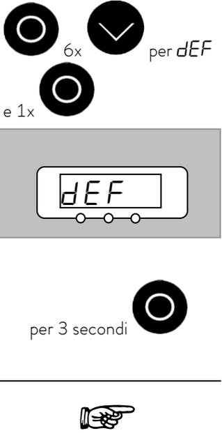
The diagram illustrates the process of restoring factory settings. It shows three stages: 1) Pressing the 'DEF' button 6 times, with the 'DEF' menu appearing on the display. 2) Pressing the 'DEF' button once, with the display showing 'DEF' in a flashing state. 3) Pressing the 'DEF' button for 3 seconds, with the display showing 'done' and returning to the temperature display. A hand icon points to the 'done' confirmation.
