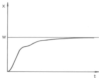
Fig. 35: Control parameters  $T_n$  and  $T_v$  too large
