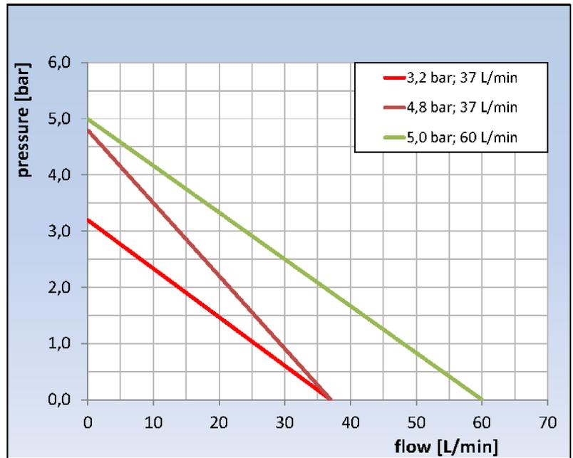
Fig. 71: Characteristic curves of the pumps
