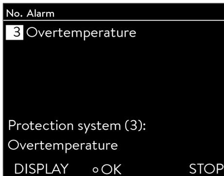
Fig. 68: Overtemperature alarm
