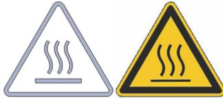
A "Hot surface" graphical symbol is affixed to the device. This symbol warns against hot surfaces on the device. These surfaces must not be touched during operation. These surfaces must be allowed to cool to room temperature before they can be touched during other operation phases such as servicing.
