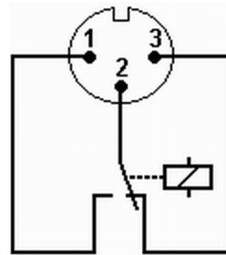
Fig. 7: Flange plug (front) in fault condition
