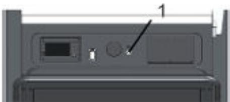
Fig. 54: Main battery switch
