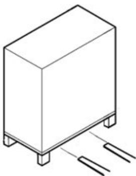
1. Only insert the forks of the industrial truck into the wider side of the device.
