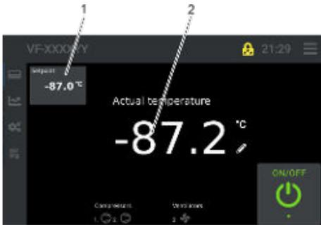
Fig. 116: Cooling chamber temperature set point icon
