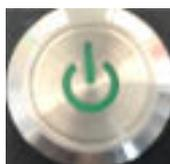
Fig. 12: Main battery switch not pressed
