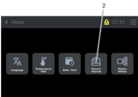
Fig. 34: Settings\_Record interval
