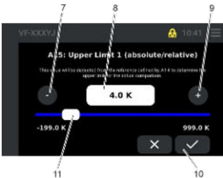
Fig. 114: Alarm message A15\_Changing the limit value
