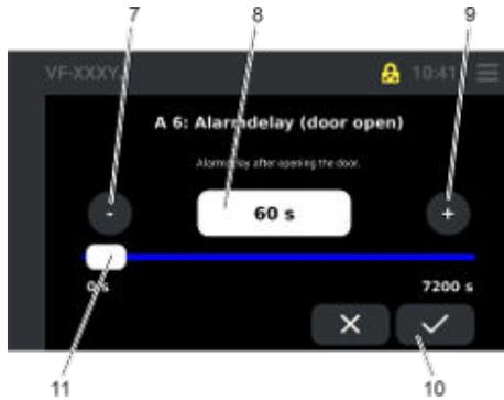
Fig. 100: Alarm message A6\_Changing the setting value
