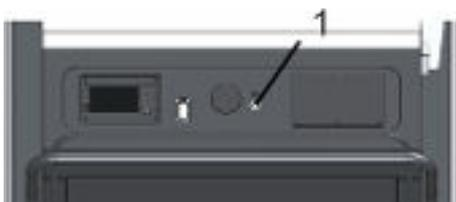
Fig. 48: Main battery switch
