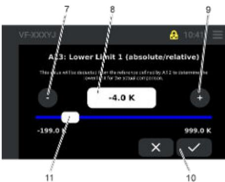
Fig. 107: Alarm message A13\_Changing the limit value
