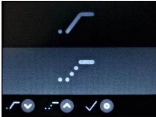
Use keys ① and ② to switch between the two start options. The chosen option is marked in gray and is confirmed with key ③. The display returns to the menu basic settings. The symbol of the selected start option is always shown together with the symbol of the operation time in the input and display windows.
