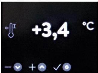
The switch-on point for the over-temperature alarm can be set between 0.0 K and +10 K above the set point temperature. The switch-on point for the under-temperature alarm can be set between 0.0 K and -10 K below the set point temperature. Only if process-related and absolutely unavoidable, should the value for the under-temperature alarm be set lower than -4.0 K and the over-temperature alarm to values lower than +2.0 K.
