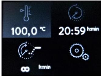
Keys ① and ② permit to move in the menu. The current function is marked in gray and can be opened with key ③. If the saved set points below the function symbols are in conformity with your process requirements, the Water Bath can be started by pressing key ④ (keep pressed for 3 seconds) and switched off again by pressing key ④ (shortly).
