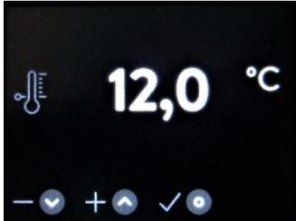
The maximum set point can be defined between 10.1 °C and 100 °C, the minimum set point between 10.0 °C and 99.9 °C. The values of both functions are interlocked. The maximum limitation of the set temperature cannot be set lower than the minimum limitation and vice versa. Therefore, the temperature can be set and limited between 10 °C and 100 °C.
