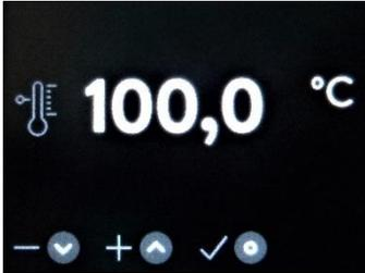
Use keys ① and ② to set the required temperature value, confirm with key ③ and return to the main menu. The set point is now displayed beneath the temperature symbol in the main menu.
