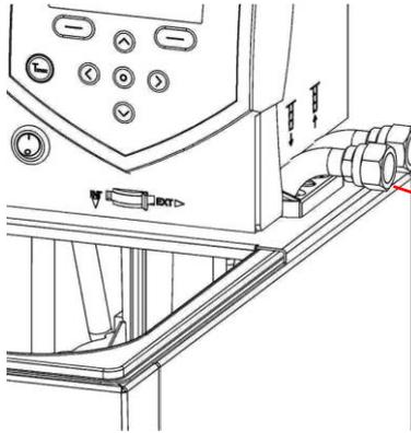
To ensure the greatest volume flow, with operation as a circulation thermostat ensure the shortest possible hose connections with the largest possible hose internal diameter.
