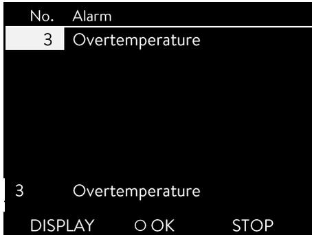
When the bath temperature is located above the overtemperature switch-off point, a two-tone alarm sounds. "Overtemperature" appears in the display, the heater switches off on all poles and the pump and chiller are switched off via the electronics.
