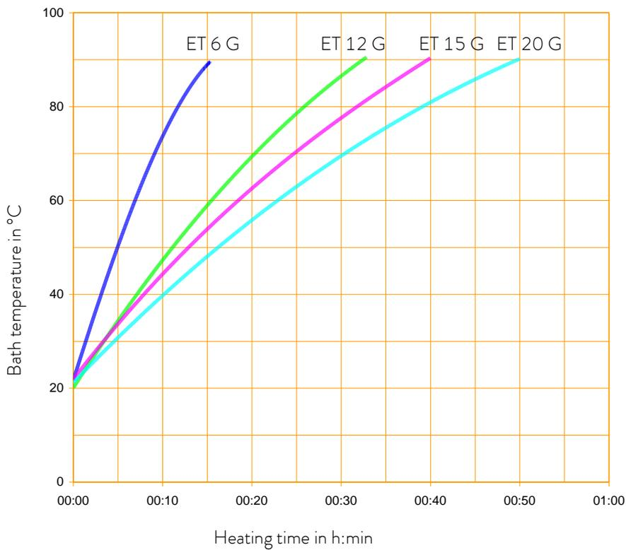
Heating curve for ECO GOLD heating thermostats with stainless steel bath
