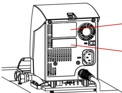
Upper module receptacle (approx. 51 mm x 27 mm) for RS 232/484 module / analog module / contact module / Profibus module
