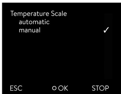
With **Temperature Scale** you can define the scaling of the y axis (temperature value).
