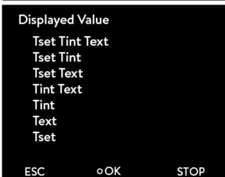
With display **Measurements** you can define which temperature values are to be graphically displayed.
