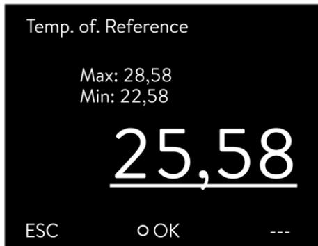
The entry window appears. The value indicated on the reference thermometer must be entered as the value.
