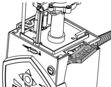
The cooling coil can only be mounted on one side of the control head. This is located on the side with the mains switch.
