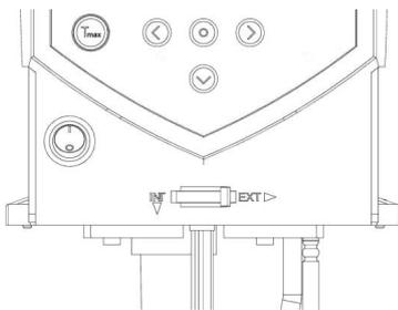
Switch the button for the distribution of the pump flow to “EXT”.
