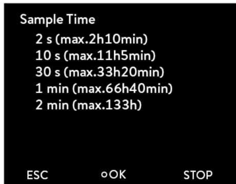
With **Rec. Interval** you define the time interval between recorded temperature measurements (the values in brackets state the maximum recording time).
