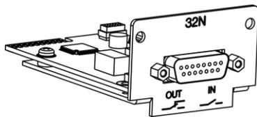
Contact module (catalogue no. LRZ 915) with 15-pole D-sub socket. Range of functions as LRZ 914, but with three relay contact outputs (changeover, max. 30 V/0.2 A) and three binary inputs for control via external voltage-free contacts.
