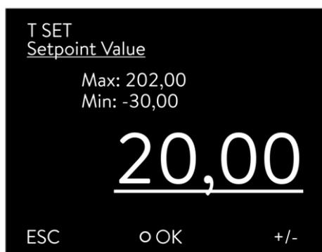
The entry window appears. The cursor below the temperature value flashes and can be changed within the displayed limits.
