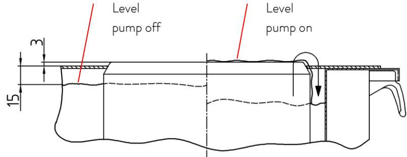
Recommendation for the adjustment of the cylindrical working chamber
