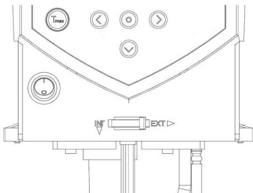
With a pure bath application, the selector switch has to be set to **INT**.
