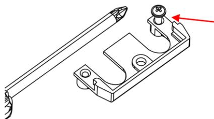
Cut the thread with the screw
