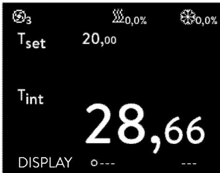
In the softkey bar, the middle softkey, "Menu", and the softkey on the right, "Standby", are hidden. The functions associated with them are no longer available.
