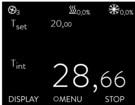
The current bath temperature ( $T_{int}$ ) is displayed with the status display above it, the expanded status display at the top margin and the soft-key bar at the bottom margin.
