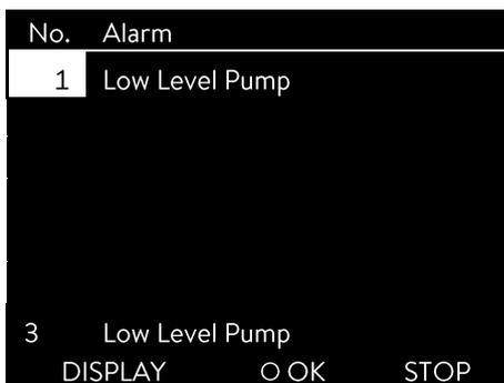
When the liquid level falls so far that the heaters are no longer completely covered with liquid, a two-tone alarm sounds. "Low Level Pump" appears in the display, the heater switches off on all poles and the pump and chiller are switched off via the electronics.
