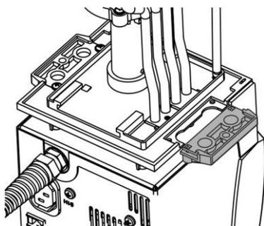
The pump connection set can be mounted on one side of the control head (see illustration).
