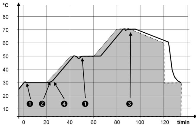
The tolerance entry can have a large effect with external bath control. The adjacent graph of the edited trace shows the possible run-on of the actual temperature in the bath vessel (continuous line) for the set-point temperature of the programmer (highlighted in gray).
