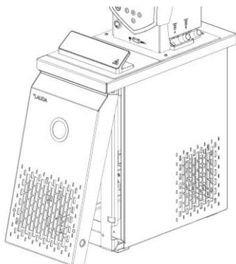
The cooling circuit is largely maintenance-free. Remove dust and contamination from the condenser at regular intervals (depending on operating period and exposure conditions).
