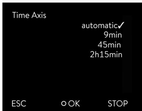
With **Time axis** you can define the temporal range over which the measurements are to be displayed.
