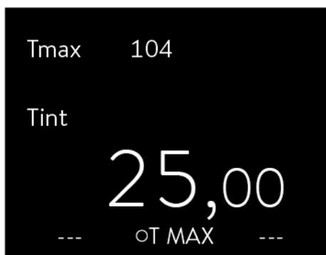
With the key  $T_{max}$  you check or change the overtemperature switch-off point:
