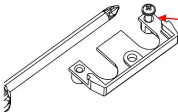
Cut the thread with the enclosed screw
