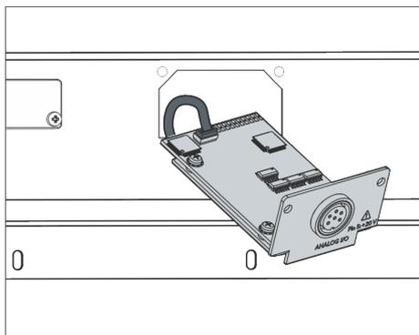
Fig. 4: Connecting the interface module (schematic diagram)
