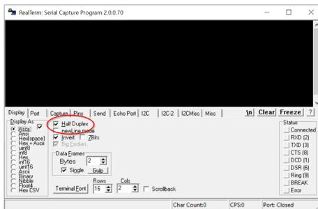
Fig. 12: Setting the transmission type
