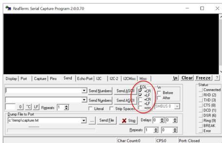
Fig. 13: Setting command lines to end automatically with CR/LF
