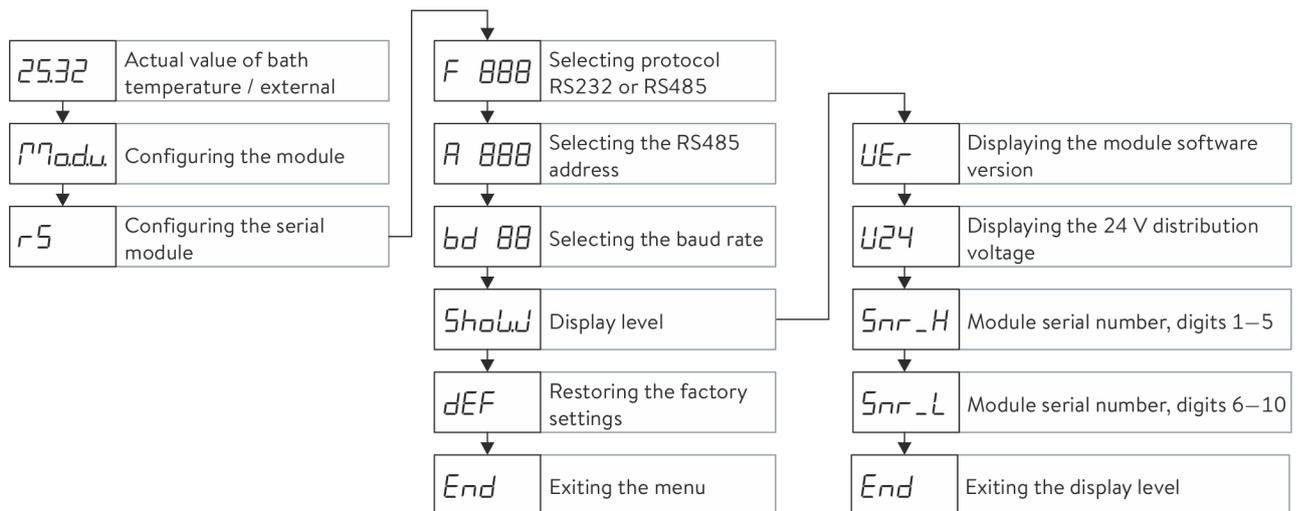
Fig. 10: Menu - RS 232/485 interface to Master operating unit
