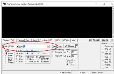
Fig. 11: Example in RealTerm: selecting the baud rate and COM port
