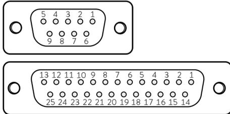
Fig. 7: D-Sub socket contacts, 9 and 25-pin
