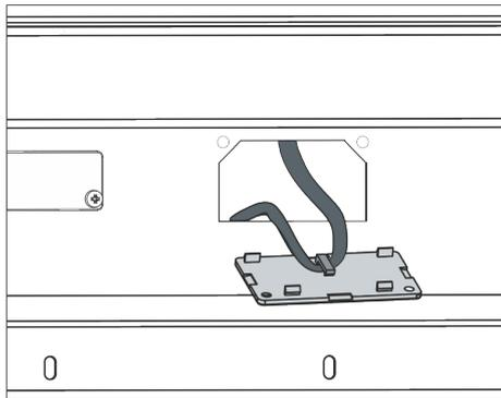
Fig. 3: Detaching the LiBus ribbon cable (schematic diagram)
