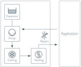
The cold oil flooded flow system with a small active volume guarantees dynamic cooling and heating, even in the most demanding applications.
