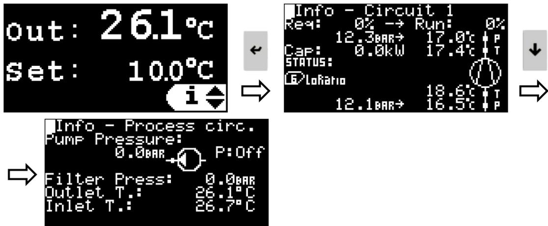
**Refrigerant compressor control and temperature stability:** The chiller relies in its ability to adjust the compressor speed to match the cooling capacity required by the application to maintain a high water outlet temperature stability.
