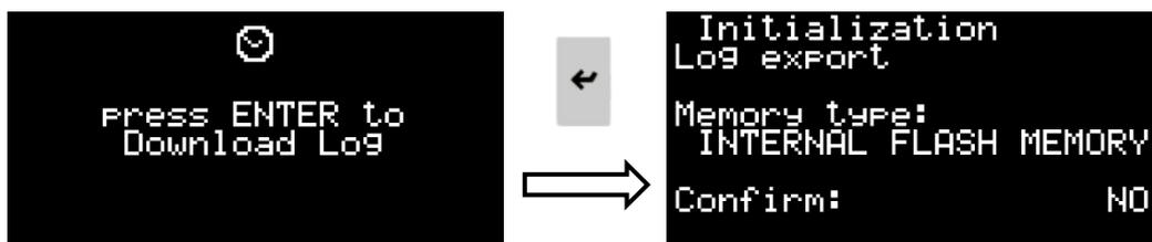
2. Press **Enter** and then the **Up** or **Down** buttons to select where to save the log file. The file can be stored in the chiller's controller Internal Flash Memory or it can be saved to a connected USB drive.
