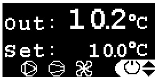
The main screen shows the current outlet temperature, the current setpoint and it shows which motors in the chiller are currently running.
