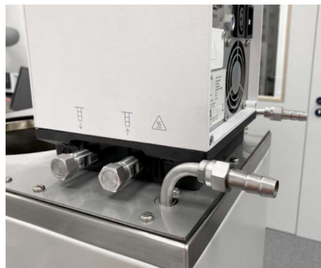
Figure 3: Universa MAX connected to the UB 40 J base and split cooling coil connections
