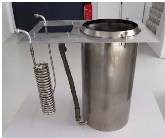
Figure 1: Cylinder of the bath lower section with new bath bridge and installed cooling coil
