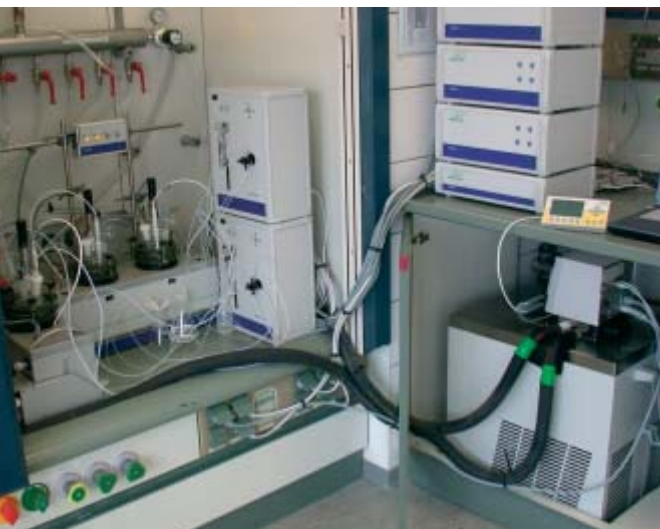
The synthesis reactor system with connected LAUDA RP 855 C cooling thermostat
