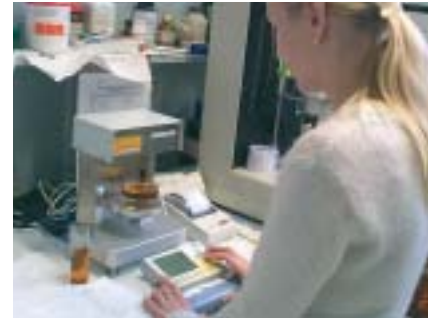
LAUDA measuring instruments, such as the ring / plate tensiometer TD 2 (photo) are used by Siemens for determining the surface tension, for example.
