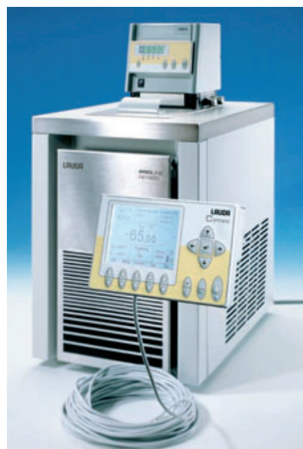
Fig. 3: Lauda Proline cooling thermostat with removable operating unit
