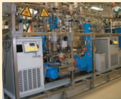
Combination of LAUDA process thermostats Integral T with LAUDA cooling thermostats RE 307 for flexible cooling of the polymer suspensions.
