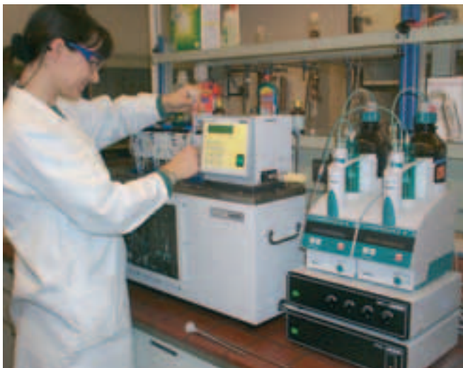
Viscosity measurement with the LAUDA PVS in transparent thermostats
