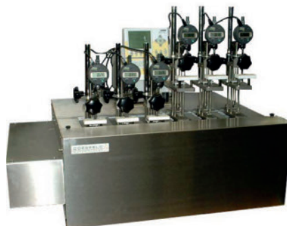
Fig. 1. Basic Vicat/HDT system with six test stands and digital measurement points. A digital thermostat ensures precise test temperatures in the bath medium
