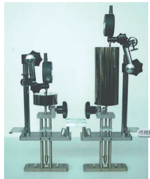
Fig. 2. Adjusting the stand for method A (10 N) and method B (50 N). Test instrument with mounted thermoplastic samples in the lower region of the diagram, side view
