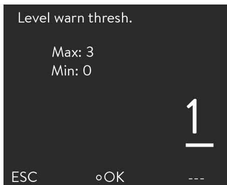
Fig. 43: Specifying the Alarm level
