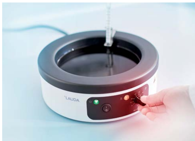
Round bath with a diameter of 200 mm and a usable depth of 50 mm
